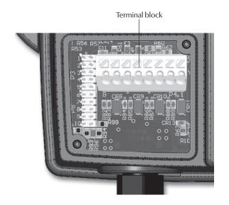
Open the front panels of both in.xtend boxes. Insert a CAT5E cable in the strain relief of each in.xtend box.
