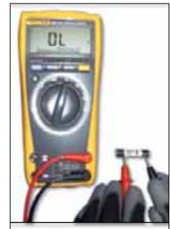
A FUSE WITH THE METER READING "BAD"
