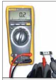
A FUSE WITH THE METER READING "GOOD"
