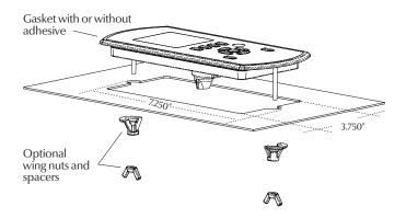
To install the in.k600 $^{\text{TM}}$  low profile, use the drilling template provided in this section. Determine the mounting location and stick the template on chosen location. The user must cut out a rectangular shape opening of 7.250 $^{\text{TM}}$  by 3.750 $^{\text{TM}}$  according to the template (see illustration).
